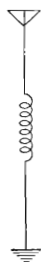
Fig. 40. Improved crystal receiver, using an antenna coupler. This set will tune sharper than that of Figure 22.
