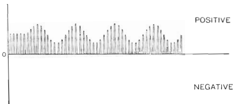
Fig. 32. Graph showing flow of pulsating direct current through the crystal detector. Note the action of the detector.
