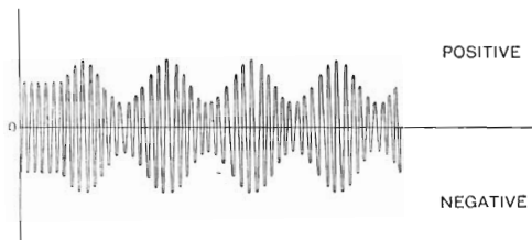
Fig. 30. Wave form of alternating current set flowing in the aerial-ground system when the modulated radio wave shown in Figure 29-C passes across the aerial of the receiving set.
