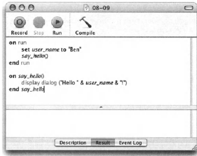
Figure 8-9. The run handler, which was implied in the last script, is described explicitly here.
