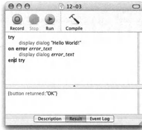
Figure 12-3. Trapping the Cancel button error using the try block
