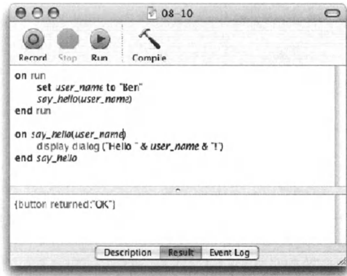
Figure 8-10. Passing the user_name variable to the say_hello handler
