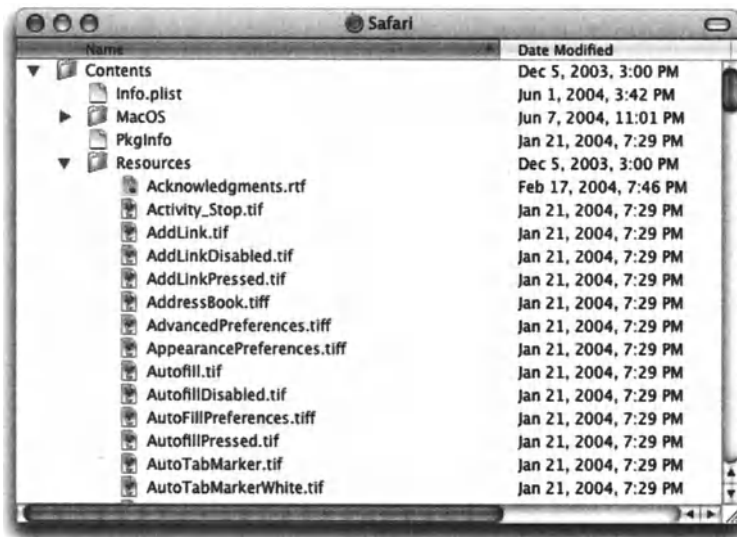
Figure 13-4. The open package of the application Safari
