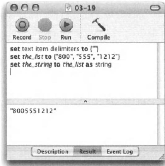
Figure 3-19. When the text item delimiters property is set to an empty string, the list items just squish together.
