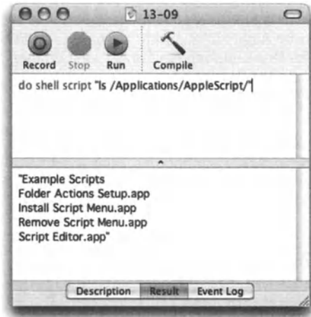
Figure 13-9. The ls command passed using the do shell script command from the Script Editor. The parameter passed along with the ls command is a POSIX path pointing to the AppleScript folder in the Applications folder.
