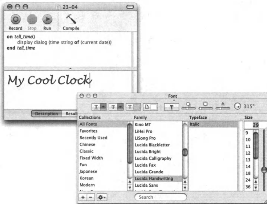
Figure 23-4. You can add formatted text to the description pane in the Script Editor script window. This text will be displayed when the script application starts up.
