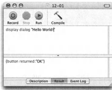
Figure 12-1. The script shows the simple display dialog command. The Result tab in the lower split view shows the record AppleScript returned once the user clicked OK.
