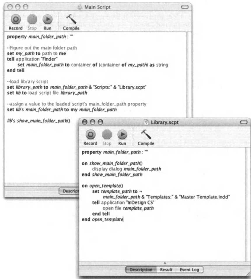
Figure 18-2. The two scripts used by the system: the main application script called Main Script and the loaded script called Library.scp
