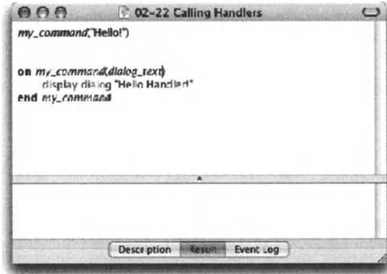
Figure 2-22. When the handler my_command is called, the variable dialog_text in the handler is going to be replaced with the text “Hello!” from the handler call line.
