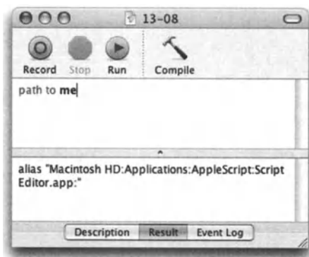
Figure 13-8. The path to me command in Script Editor returns the path to the Script Editor application.
