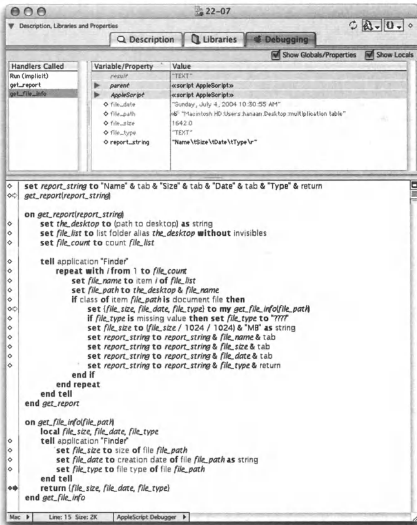
Figure 22-7. Script Debugger's script window in AppleScript Debugger mode
