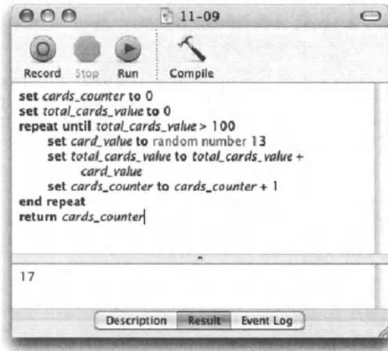
Figure 11-9. Repeating until the total card value reaches over 100
