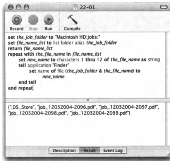
Figure 22-1. The return command stops the script and places the value of the file_name_list in the result panel in Script Editor.
