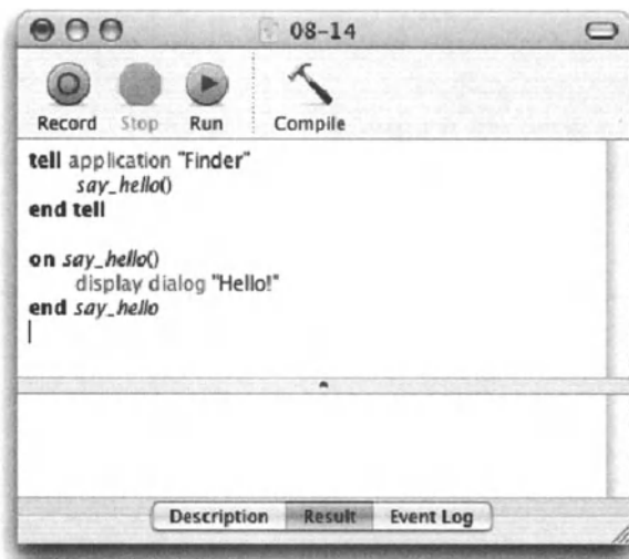
Figure 8-14. Calling a handler from within the Finder tell block returns an error.
