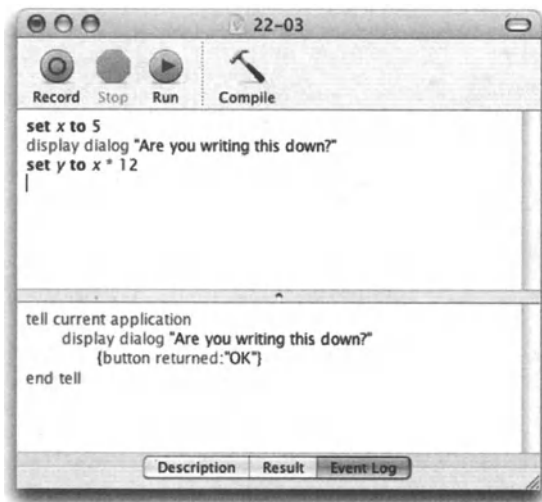
Figure 22-3. A simple script and the results that the event log has captured
