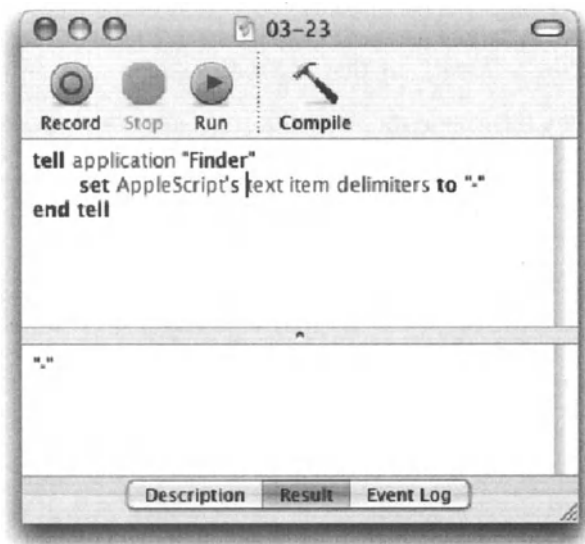
Figure 3-23. Setting the value of the text item delimiters property inside an application tell block
