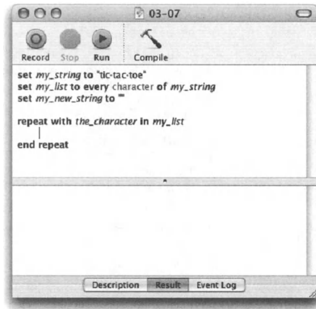
Figure 3-7. The variables are defined and a repeat loop skeleton has been created.
