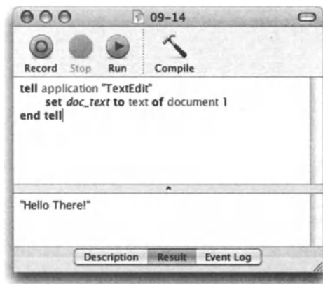
Figure 9-14. The text of a TextEdit document is assigned to a variable, but AppleScript returns the result as a string.
