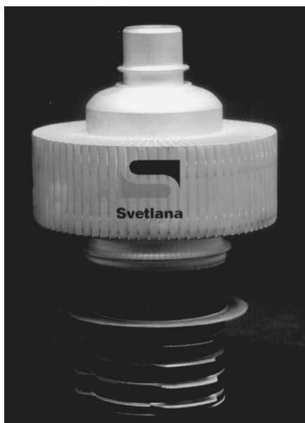
FIGURE 3.14 5CX1500B power pentode device. (Courtesy of Svetlana Electron Devices, Huntsville, AL.)
