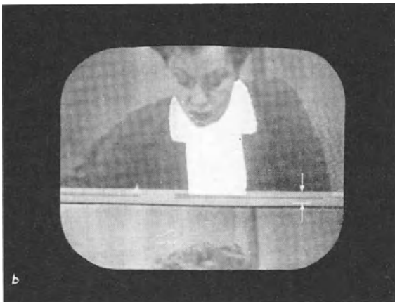
Fig. 19-31 Oscillogram with normal picture modulation. a ) one vertical pulse; b ) one horizontal pulse; c ) and d ) voltage waveforms of single lines
