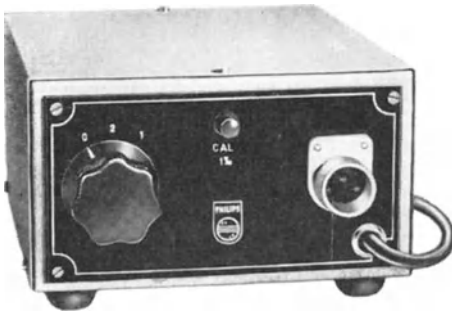
Fig. 31-6 Exterior of the Philips unit "PT 1205" according to the layout in Fig. 31-5
