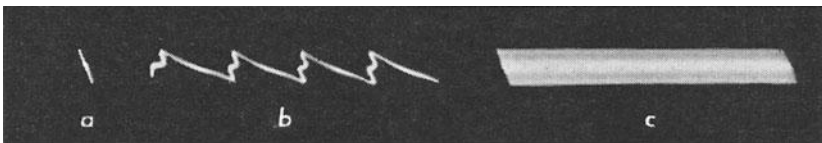
Fig. 3-14 Effect on the screen produced by magnetic interference
