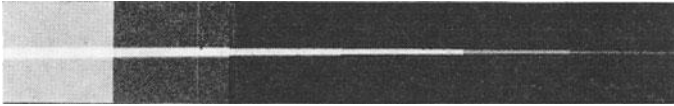
Fig. 32-24 Influence of duration of exposure on the line thickness of the oscillogram trace at enlarging
