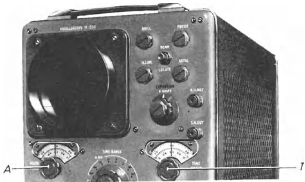
Fig. 7-21 Marconi oscilloscope TF1330. Oscillogram interpretation by means of calibrated picture shift A Shift of pattern in Y -direction, amplitude measurement T shift of pattern in X -direction, measurement of time scale
