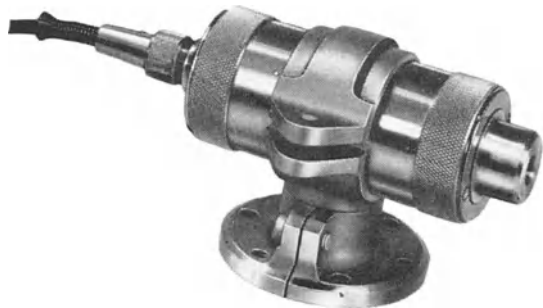
Fig. 30-11 "PR 9260" Absolute pickup. a ) Fixed for observation of vertical oscillations; b ) as a ) but for horizontal oscillations
