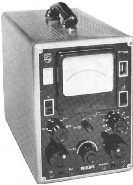
Fig. 31-10 Philips "PT 1200" carrier frequency measuring bridge
