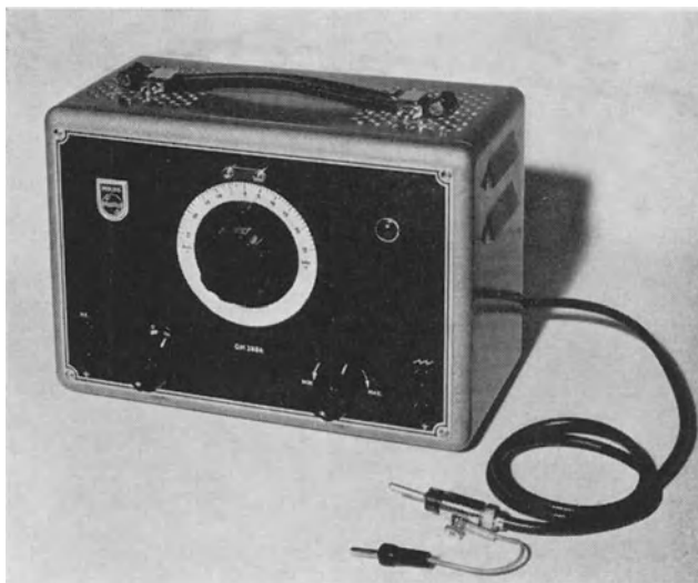
Fig. 18-6 Exterior of "GM 2886" Frequency Modulator; central scale for detuning fundamental frequency of 4 Mc/s by \pm 25 kc/s
