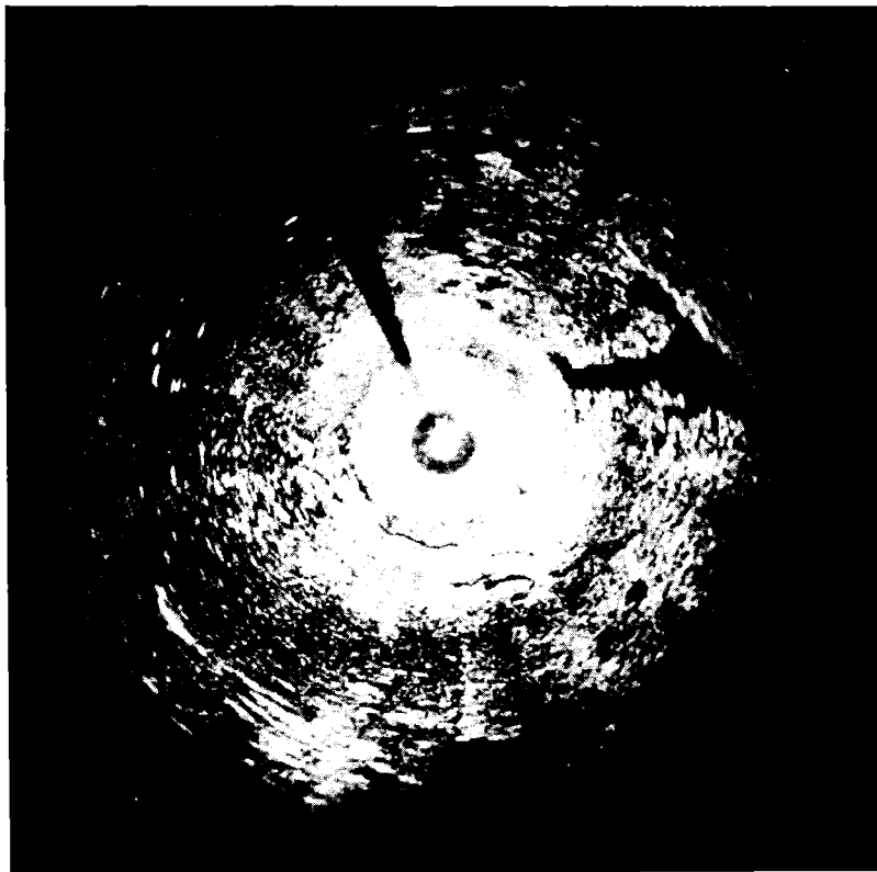
FIG. 3-28.—The Kanto plain north of Tokyo. Wavelength = 3.2 cm, 3° beam, altitude 10,000 ft, radius 28 nautical mi. 35°59'N. 139°59'E.
