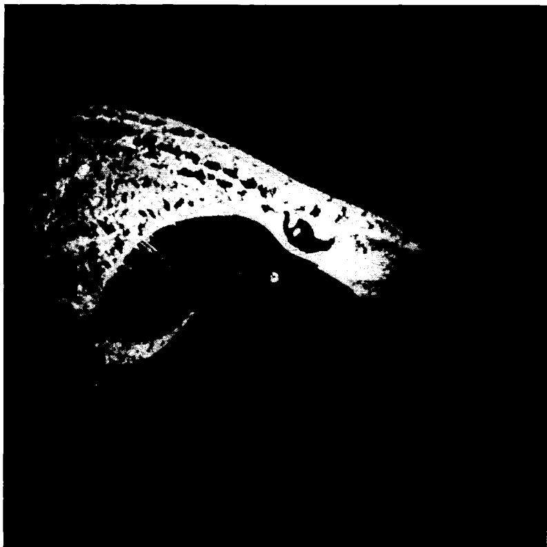
FIG. 3-19.—Tip of Cape Cod, Mass., with Provincetown Harbor. Wavelength = 1.25 cm, 0.8° beam, altitude 4000 ft. radius 3 nautical mi. 42°03'N. 70°06'W.
