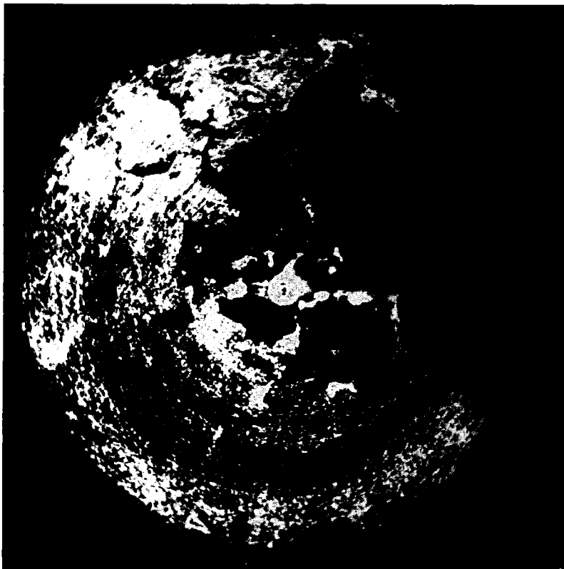
FIG. 3-33.—Outer harbor, Boston, Mass. Wavelength = 1.25 cm, 0.8° beam, altitude 8000 ft, radius 10 nautical mi. 42°18'N, 70°58'W.
