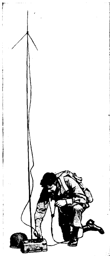
FIG. 8-5.—The AN/PPN-2 beacon. The AN/PPN-2 is a 1.5-m beacon designed for use principally by paratroops.
