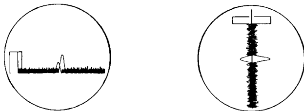
(a) Side-by-side presentation (K-scope). Signal return from the right lobe is the stronger.
