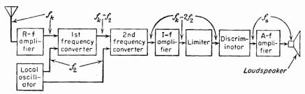
Fig. 12-28. A block diagram of an f-m receiver.
