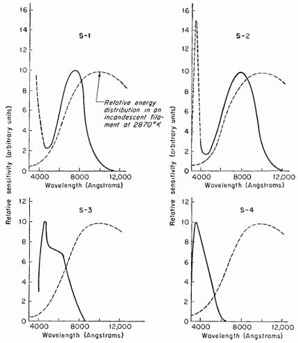
Fig. 15-10. Standard RMA spectral-response curves.
