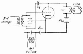
Fig. 12-9. A grid-bias-modulated class C amplifier.
