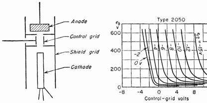
Fig. 13-16. Typical electrode structure for a shield-grid thyratron.
