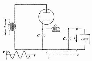
Fig. 5-6. A half-wave rectifier with a filter.
