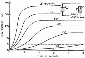
Fig. 16-6. Current vs. time curves for six values of the battery voltage in the circuit shown in the insert. (Courtesy of Bell Loboratories.<sup>2</sup>)
