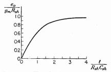
Fig. 7-31. The rise in output voltage with time in the circuit of Fig. 7-30.
