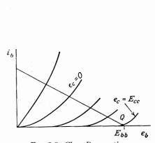
Fig. 8-3. Class B operation.
