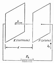
Fig. 3-4. Diode with parallel plane electrodes.
