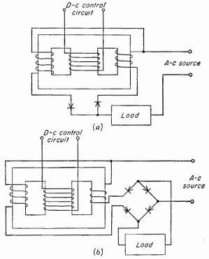
Fig. 16-24. Magnetic-amplifier circuit for (a) a-c loads, (b) d-c loads.
