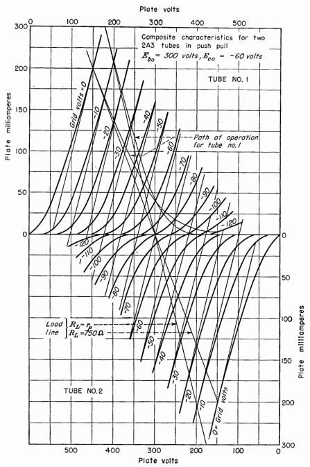
Fig. 8-21. Composite characteristics for two 2A3 tubes in class AB<sub>1</sub> push-pull.
