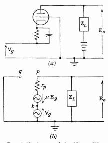
Fig. 7-58. A grounded-grid amplifier.
