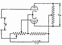
Fig. 7-9. A balanced voltage amplifier.
