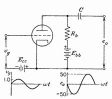
Fig. 5-9. A triode voltage amplifier with fixed grid bias.
