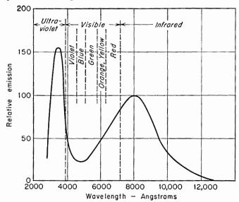
Fig. 15-4. Spectral-sensitivity curve for a typical cesium-cesium oxide-silver cell. emitted electrons. Figure 15-5 shows a picture of several cells. In most photocells the cathode is a semicylindrical surface so arranged that light falls on its concave face. The anode is a straight wire running along the axis of the cylinder.
