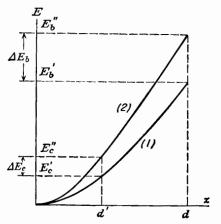
Fig. 4-2. Potential distribution in a diode for two values of plate voltage. Electrons have zero initial velocity.
