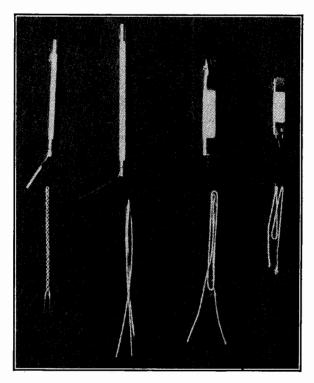
${\rm Fig.}$  2-6. Indirectly and directly heated cathodes used in high-vacuum receiving tubes.
