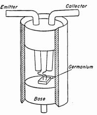
Fig. 16-13. Cutaway view of a transistor.
