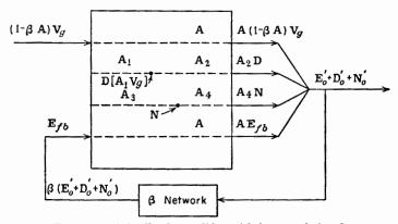
Fig. 10-4. A feedback amplifier with increased signal.
