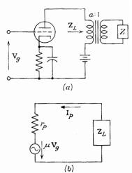
Fig. 8-5. (a) A power amplifier. (b) Its linear equivalent circuit.
