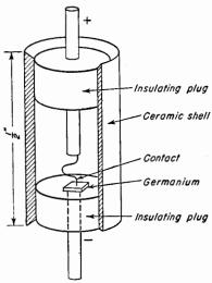
Fig. 16-8. Construction of a germanium diode.
