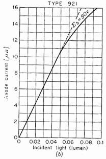
Fig. 15-7. Variations of emission current with light flux for (a) a vacuum-type cell, (b) a gas cell.
