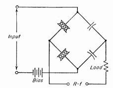
Fig. 16-30. A practical circuit for a dielectric amplifier.
