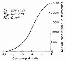
Fig. 12-26. Variation of  $g_m$  with grid bias for a 6SJ7.
