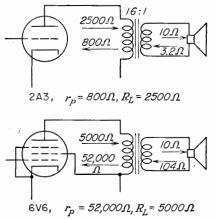
Fig. 8-16. A loudspeaker is damped by the power tube if the tube's output impedance is low.
