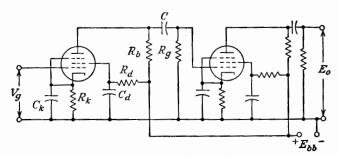
Fig. 7-11. An R-C-coupled pentode amplifier.
