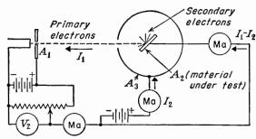
Fig. 2-9. Tube for measuring secondary-emission effects.
