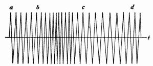
Fig. 5-2. Angle-modulated wave.
