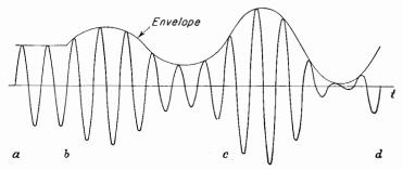
Fig. 12-1. Various degrees of amplitude modulation.
