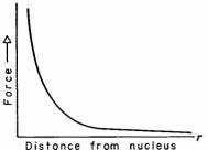
Fig. 2-1. Force on an electron in the vicinity of an isolated nucleus.
