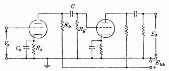
Fig. 7-10. An R-C-coupled triode amplifier.
