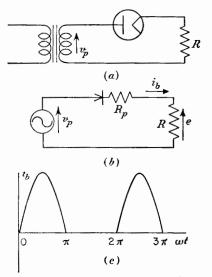
Fig. 14-3. (a) Circuit diagram for a half-wave rectifier with resistance load. (b) Equivalent circuit for (a) using a high-vacuum diode. (c) Waveform of load current.
