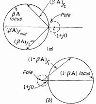
Fig. 10-22. Determination of the stability of the amplifier of Fig. 10-6. (a) The  $\beta A$  diagram. (b) The 1- $\beta A$  diagram.
