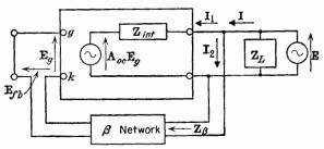
Fig. 10-10. Testing a voltage-feedback circuit for output impedance.
