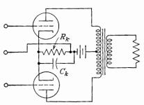
Fig. 8-23. A push-pull amplifier employing cathode bias.
