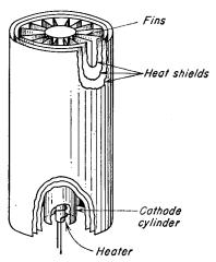
Fig. 13-7. A heat-shielded cathode.
