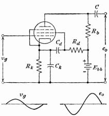
Fig. 5-12. A pentode voltage amplifier.
