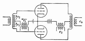
Fig. 12-12. Basic circuit for a balanced modulator.
