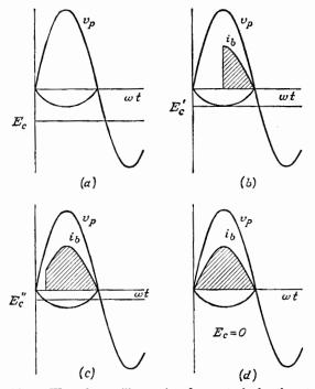
Fig. 14-24. Waveshapes illustrating d-c control of a thyratron.
