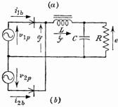
Fig. 14-19. (a) A full-wave rectifier with an L-section filter and a resistance load. (b) Equivalent circuit for (a).
