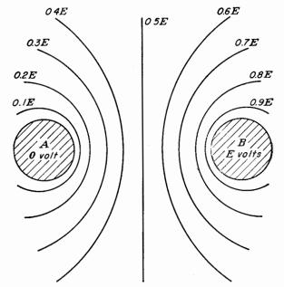
Fig. 1-3. The potential field between two parallel cylinders.
