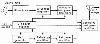
Fig. 5-3. An a-m transmitting system.
