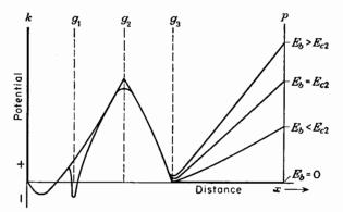
Fig. 4-20. Potential distribution in a pentode.
