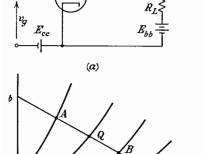
Fig. 8-1. (a) A power amplifier with direct-connected load. (b) The load line for this amplifier.
