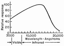
Fig. 16-18. Spectral response of a selenium photoconductive cell.
