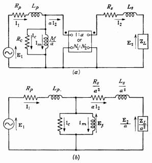
Fig. 7-65. Equivalent circuits for a power transformer.
