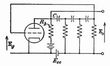
Fig. 11-19. A phase-shift oscillator.
