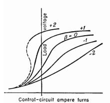
Fig. 16-26. Effects of negative and of positive feedback with magnetic amplifiers. ( $|\beta| \propto \text{No. feedback turns.}$ )
