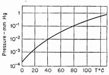
Fig. 13-8. Vapor pressure of mercury as a function of temperature.
