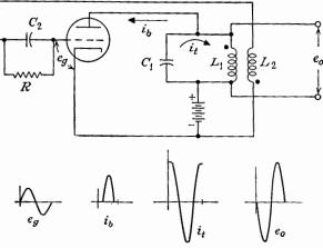
Fig. 5-20. A feedback oscillator.
