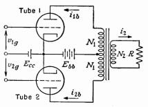
Fig. 8-17. A push-pull amplifier using fixed bias.
