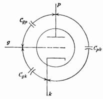
Fig. 4-13. Interelectrode capacitances in a triode.
