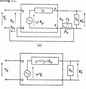
Fig. 10-17. Equivalent circuits for the amplifier of Fig. 10-16.
