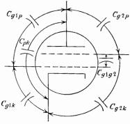
Fig. 4-15. Interelectrode capacitances in a tetrode.
