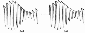
Fig. 12-16. e<sub>o</sub> is the envelope of the modulated r-f waveform unless clipping occurs.
