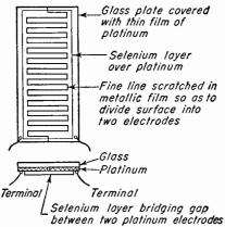
Fig. 15-1. Construction of a photoconductive cell.
