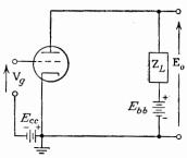
Fig. 7-1. A grounded-cathode grid-driven plate-loaded amplifier.
