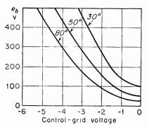
Fig. 13-14. Firing characteristics for a type FG27A thyratron showing the effects of temperature change.
