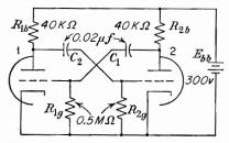
Fig. 11-23. An alternate representation for the multivibrator.
