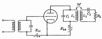
Fig. 9-1. Basic circuit for a tuned power amplifier. (Neutralization not shown.)
