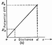
Fig. 1-7. Potential distribution between parallel plane plates.
