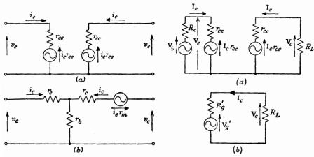
Fig. 16-16. Equivalent circuits for transistors.
