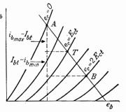
Fig. 8-8. Distortion occurs if AT is not equal to TB.
