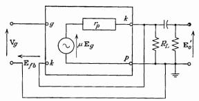
Fig. 10-14. An equivalent circuit for the cathode follower showing the feedback arrangement.
