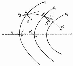
Fig. 1-14. Focusing action of the electric field in an electron lens.
