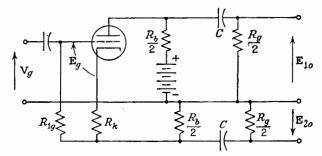
Fig. 7-48. A split-load type of phase inverter.
