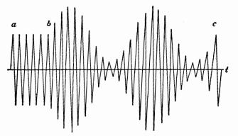
Fig. 5-1. Amplitude-modulated wave.
