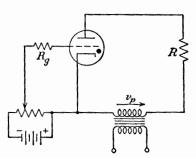
Fig. 14-23, Direct-current control of a thyratron.
