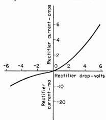
Fig. 16-11. Volt-ampere characteristic for a single copper-cuprous oxide disk.
