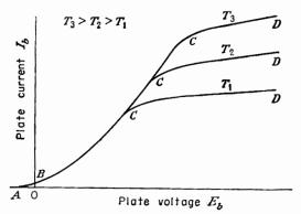
Fig. 3-3. Characteristics for a high-vacuum diode.
