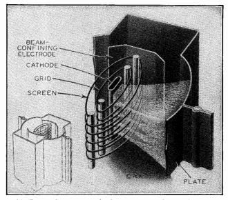
Fig. 4-29. Internal structure of a beam power tube. (Courtesy RCA.)
