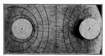
Fig. 1-6. Flux and potential field between two parallel cylinders.
