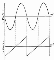
Fig. 1-17. Sinusoidal and saw-tooth waveforms.
