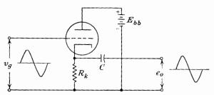
Fig. 5-18. A cathode-follower voltage amplifier.
