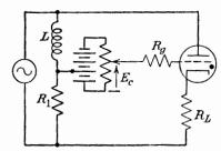
Fig. 14-31. Circuit for bias phase control.
