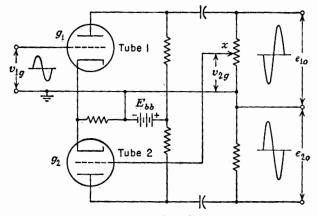
Fig. 5-16. A phase inverter.
