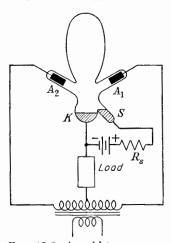
Fig. 13-9. An old-type mercury-arc tube and its circuit.
