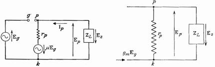
Fig. 6-21. Equivalent plate and grid circuits.
