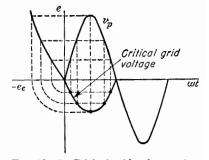
Fig. 13-15. Critical grid voltage when an alternating voltage is applied to the plate of a thyratron.
