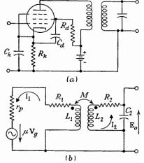
Fig. 7-81. (a) Tuned-secondary r-f amplifier. (b) Equivalent circuit of (a).
