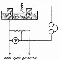
Fig. 1-2. Diagram of a potential-plotting tank.
