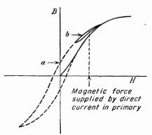
Fig. 7-66. Magnetic operation of a transformer.
