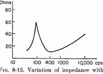
Fig. 8-15. Variation of impedance with frequency for a typical loudspeaker.
