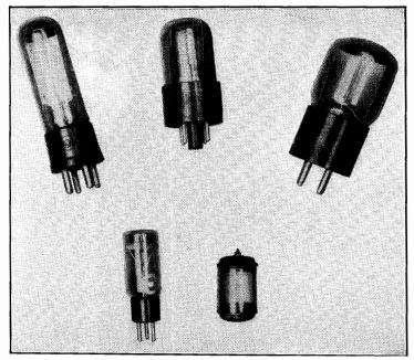
Fig. 15-5. Photoemissive cells.
