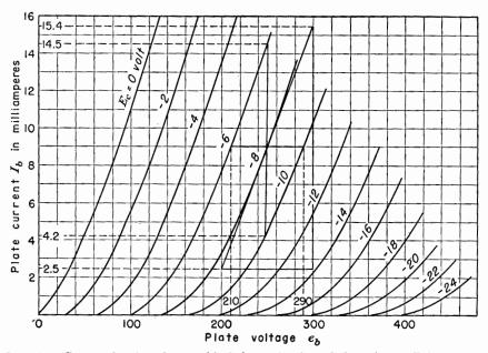
Fig. 4-9. Curves showing the graphical determination of the tube coefficients at a given operating point for a 6J5 tube.
