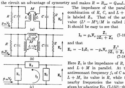
Fig. 7-84. Double-tuned r-f amplifiers. (a) Norton's equivalent circuit, (b) the circuit in  $\Pi$  form, (c) a simplified-version of the II form.
