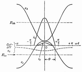
Fig. 9-3. Approximate waveforms for class C operation.
