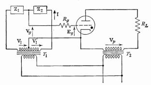
Fig. 14-27. A thyratron with phase-shift control.
