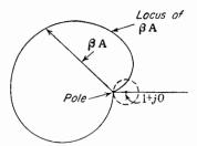
Fig. 10-23. The **GA** diagram for a transformer-coupled stage with feedback.
