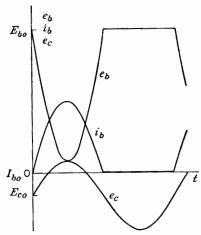
Fig. 8-4. Waveforms for class B operation.
