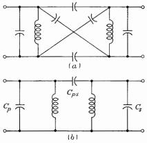
Fig. 7-63. Distributed capacitances in a transformer.
