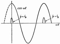
Fig. 14-22. Waveshape of the tube current for a half-wave rectifier with a II-section filter.
