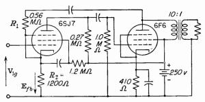
Fig. 10-20. A two-stage feedback circuit.
