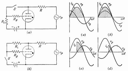
Fig. 14-25. On-off control of a thyratron.
