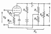
Fig. 10-6. An amplifier with simple voltage feedback.
