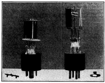
Fig. 3-1. Radio-receiver-type diodes.
