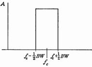
Fig. 7-75. The response of an r-f amplifier should be like this.
