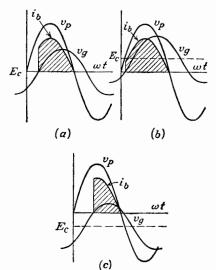
Fig. 14-32. Waveshapes for bias phase control.
