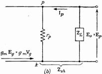
Fig. 7-2. Low-frequency equivalent circuits.
