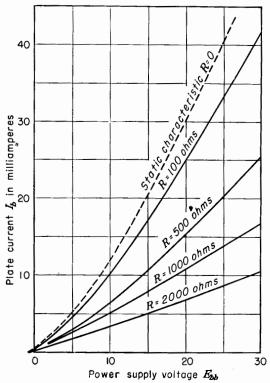
Fig. 3-12. Denamic plate characteristics for a type 6H6 diode with various load resistors.
