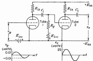
Fig. 5-10. A two-stage R-C-coupled amplifier.
