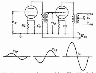
Fig. 5-11. A two-stage transformer-coupled amplifier with cathode bias.
