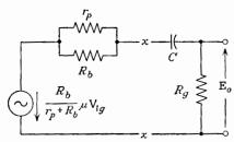
Fig. 7-18. Another Thévenin's form of the equivalent circuit of Fig. 7-17.
