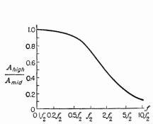
Fig. 7-24. Gain vs. frequency in the h-f range.
