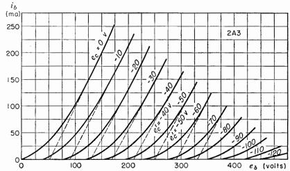
Fig. 8-20. Curves for the 2A3 tube and for the composite tube.
