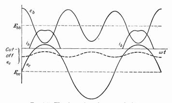
Fig. 9-7. Waveforms for a frequency doubler.
