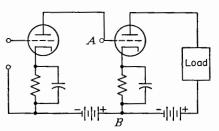
Fig. 7-6. A circuit like this will not work.
