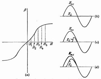
Fig. 16-23. Operation of a magnetic amplifier.
