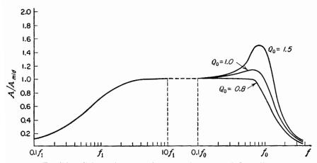
Fig. 7-71. Gain vs. frequency for a transformer-coupled amplifier.
