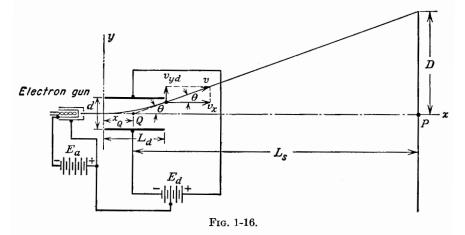
1-16. The Deflection of the Electron Beam in a Cathode-ray Tube. As an electron beam passes through the field of the electron gun, it is accelerated and leaves the gun with a velocity
