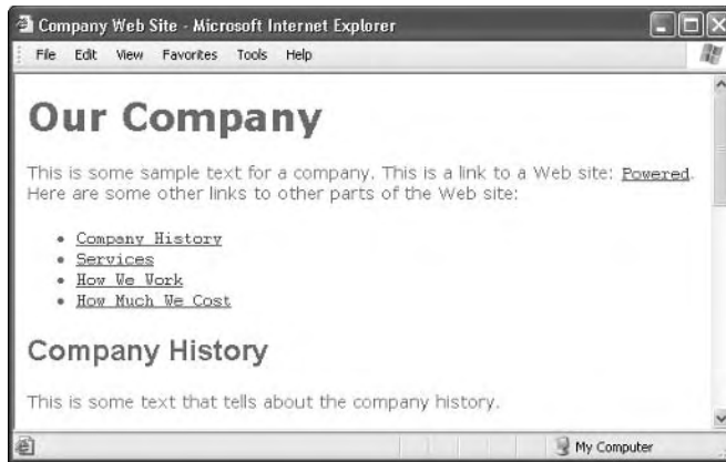
Figure 10-1: The font family for hyperlinks differs from the font family for the rest of the text.
