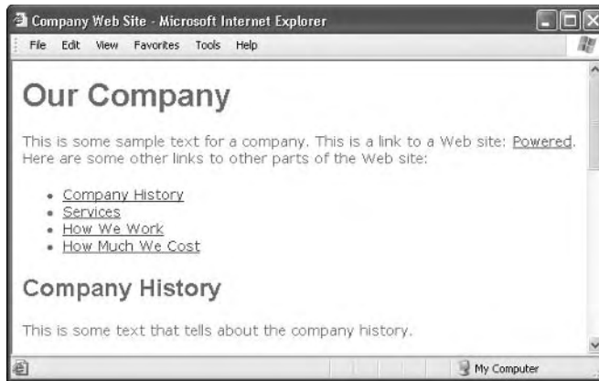
Figure 10-2: First-level headings are 24 points tall; the font size of other text is relative.
