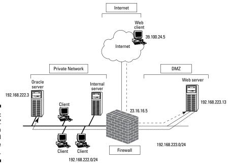
Figure 11-8: A DMZ hosting a Web-based database application.
