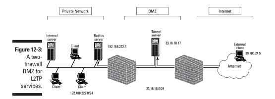
The use of public network addressing eliminates the need to define static address mappings. The external firewall allows direct access to the L2TP server using IPSec without having to readdress incoming packets.
