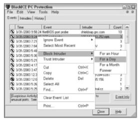
Figure 15-10: Manually block an intruder. You can specify whether the detected intrusion should cause a change in filtering at the IDS layer or at the Firewall layer.
