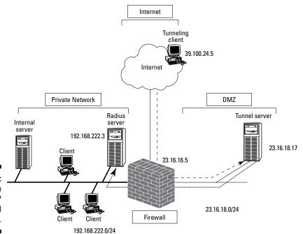
Figure 11-6: A DMZ with an L2TP tunnel server.
