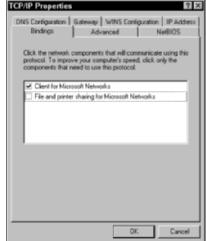
Figure 13-1: Unbind file and printer sharing.
