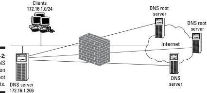
Figure 7-2: DNS resolution using root hints.
