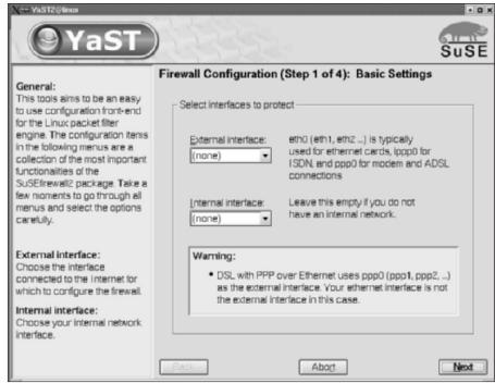
Figure 14-2: SuSEfirewall2 configuration.
