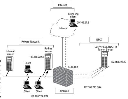
Figure 11-7: A DMZ with an L2TP tunnel server that supports NAT-T.
