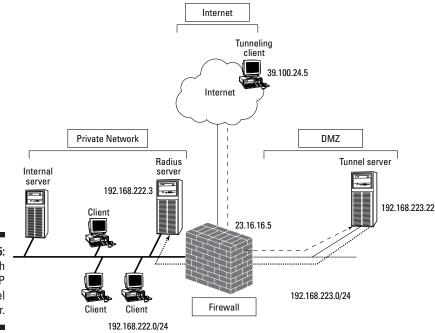
Figure 11-5: A DMZ with a PPTP tunnel server.
