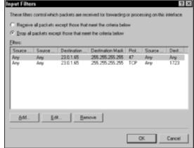
Figure 13-3: Windows 2000 input filters (PPTP).
