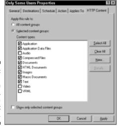
Figure 9-2: Restricting content in an ISA Server Site and Content Rule.
