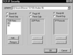
Figure 13-2: Windows NT 4.0 packet filtering.
