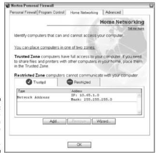
Figure 15-19: Configure zones on Home Networking tab. Click the Wizard button on the Home Networking tab to add the IP address connected to the local network adapter to the Trusted Zone. Select the Restricted tab to add addresses to the Restricted Zone.
