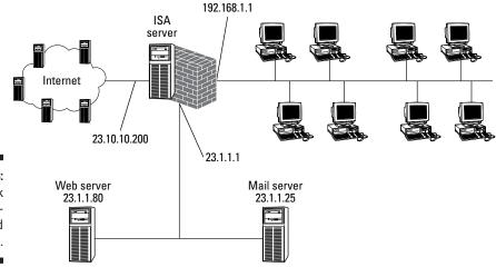
Figure 16-13: A network with a threepronged DMZ.
