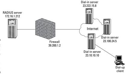
Figure 8-1: **RADIUS** provides centralized authentication.
