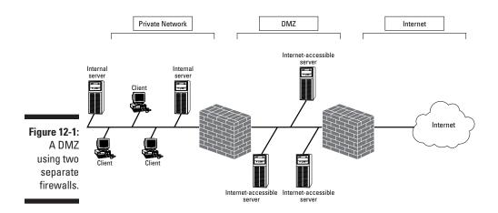
In this scenario, the two firewalls separate the DMZ from both the private network and the Internet. Although additional costs are associated with the additional firewall, this configuration is considered more secure because an attacker must breach two firewalls in order to access resources on the private network.
