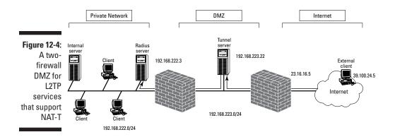
As with a PPTP tunnel server, you must first define static address mappings at the external firewall to ensure that the NAT discovery (NAT-D) and NAT-T traffic are redirected to the tunnel server in the DMZ. These static address mappings are shown in Table 12-6.
