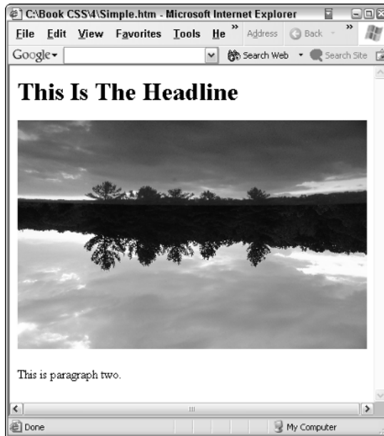
Figure 4-1: The simplest Web page design merely stacks text, pictures, and other elements on top of each other, along the left side of the page.
