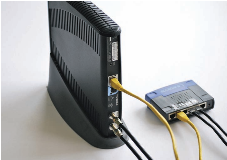
FIGURE 11-6 Modem for Internet access satellite dish system. Notice the two coaxial cables, one for receiving and one for transmitting, that come from the dish. A Category 5e cable feeds the modem output to an Ethernet hub, which is necessary because two computers are connected.
