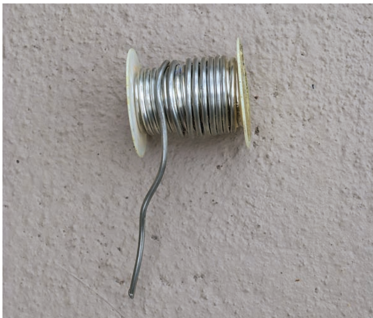
FIGURE 10-4 Wire solder for joining 12 American Wire Gauge (AWG) wire and larger.
