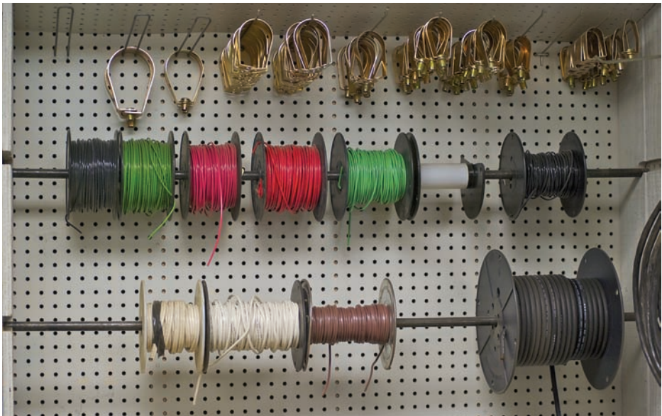
FIGURE G-4 Conductors are available in many colors, aiding in identification.
