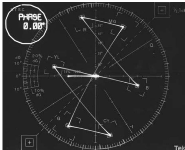
FIGURE 20.24 Vectorscope display of a color-bar signal. (Courtesy of Tektronix.)
