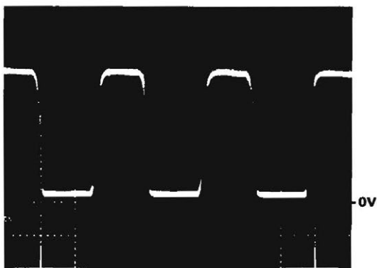
FIGURE 15 RC-type FREE-RUNNING OSCILLATOR (0, +10V power supply)
