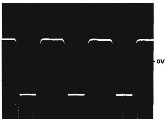
FIGURE 14 RC-type FREE-RUNNING OSCILLATOR (Using one of the filter op-amps) [-5V, +5V power supplies]
